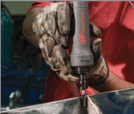
Weld cleaning and smoothing
